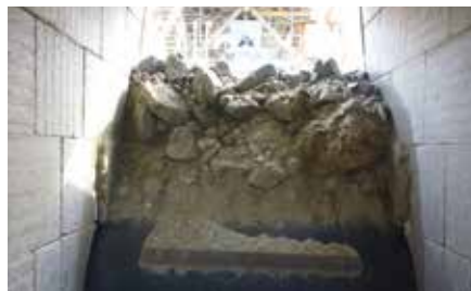
PRIMARY CRUSHED ORE 1500tph
